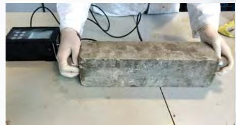
Ultrasonic Pulse Velocity (UPV) Test
