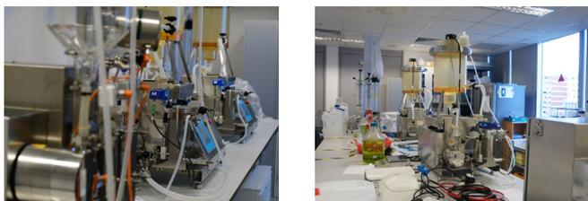
This houses equipment for purification by Tangential Flow Filtration (TFF) and gel size exclusion chromatography (SEC). The laboratory set up allows students to view demonstrations by staff as machines are centrally located and placed on laboratory benches.
