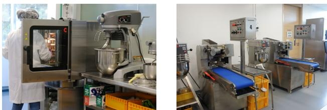
The Noodle & Snack R&D Laboratory is equipped with pilot scale equipment like semi-continuous noodle maker, combi oven, tunnel dryer, various-sized mixers to enable hands-on experience. The laboratory also provides opportunities for staff capability development to work on pre-commercial production.
