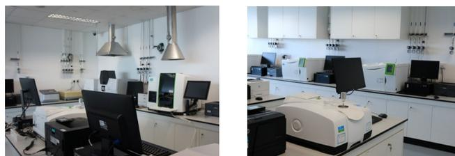
Equipped with industry-relevant equipment such as the High Performance Liquid Chromatography (HPLC) analyser, Inductively Coupled Plasma (ICP) spectrometer, and Infrared (IR) spectrometer, this laboratory is to impart hands-on skills required by industries such as forensics, petrochemical and pharmaceutical.
