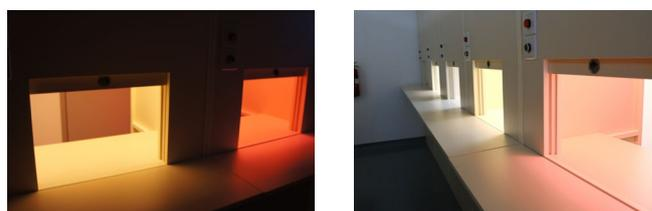
The laboratory features 10 open sensory evaluation booths, each equipped with a lighting unit of different light sources. Adjacent to the testing booths is a well-equipped sample preparation room to ensure proper sample transfer during a study. Built to conduct a range of sensory evaluation techniques, the laboratory is used to carry out studies as part of new product development or product reformulation.
