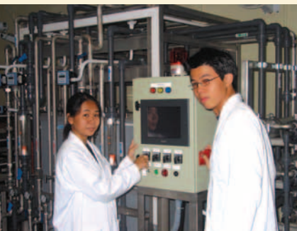
Using the UF/RO Membrane Unit to purify water
